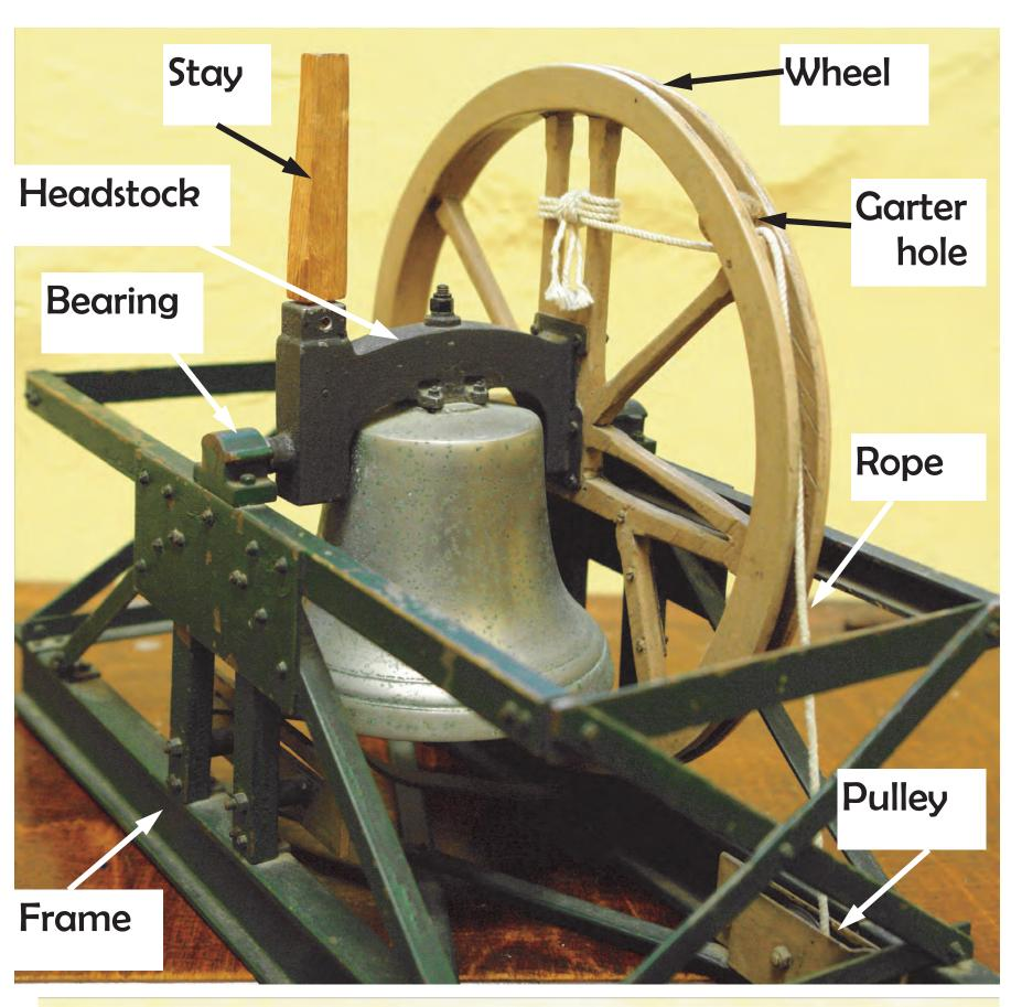
Here, the bell has been swung into the 'up' position. The stay of the bell rests against a slider underneath the bell, and the bell can be balanced mouth up.
