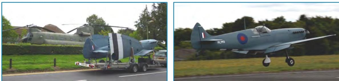
The first flight was in the hands of a test pilot at Enstone airfield in late August 2018. That flight only lasted 7 minutes because the engine overheated soon after take off. A year of modifying the cooling system and a different test pilot flew it three times in 2019. The
