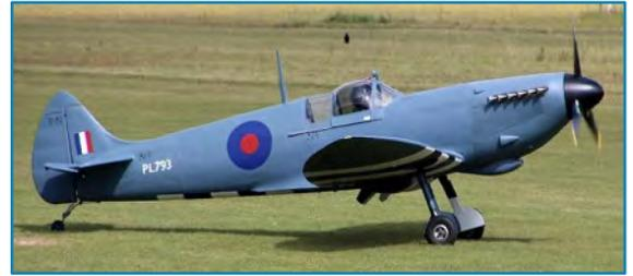
has adequate performance using a 266 horsepower V6 engine compared with the 1000 HP V12 Merlin, and uses a lot less fuel. It will cruise at 175 knots, cover 30 miles per gallon, and has enough range to go non-stop to Rome with a 45 minute reserve.
